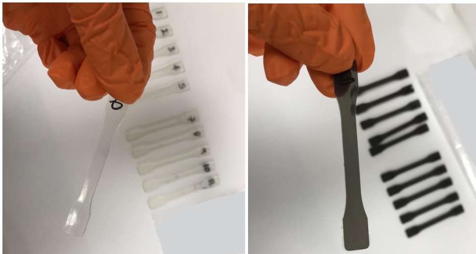
Figure 3-1: Graphene dispersed in poly lactic acid polymers (control left) and the graphene version to the right
